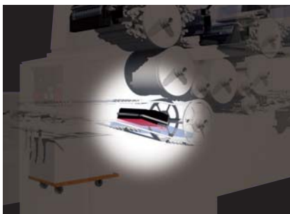
1. Ink densities and dampening solution levels are measured as sheets come out of the Truepress.
