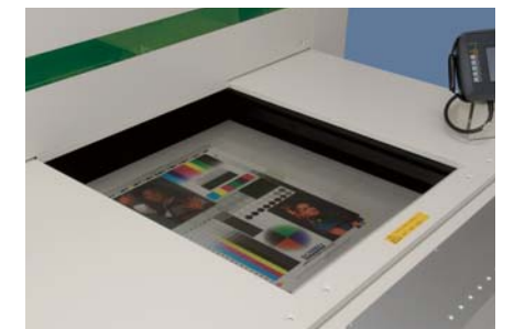
• \theta adjustment (microscopic angle adjustment) of the printing table is carried out automatically with great precision.
